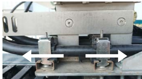
Figure 3.8 Clamps's correct direction
