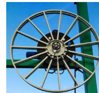
Figure 3.4 Crane position at the end of the track - Reserve number of coils wound on the mono-spiral wheel.
